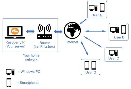
An essential task of the router is to provide a so-called **firewall**. The firewall protects the home network against unauthorised access from the Internet by blocking such access requests.
